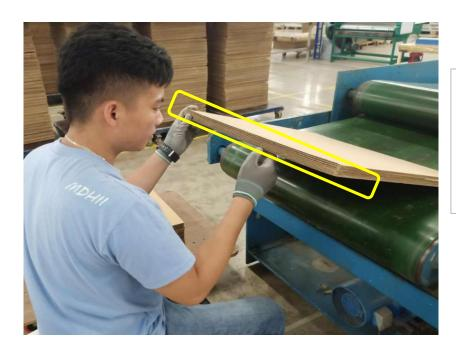
CHECK THE APEARANCE OF SHEETS (MAKE SURE THAT ALL FLUTE ARE IN ONE DIRECTION ) AND THE QUANTY OF THE LAMINATED SHEETS (3 C-FLUTE AND 5 B-FLUTE)
